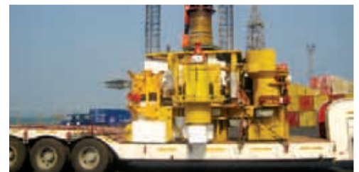
2. Subsea trees USA, Singapore, UK, Norway Supplied by FMC. The subsea trees control the production or injection of individual wells. 19 have been ordered for the Jubilee Phase 1 project.
