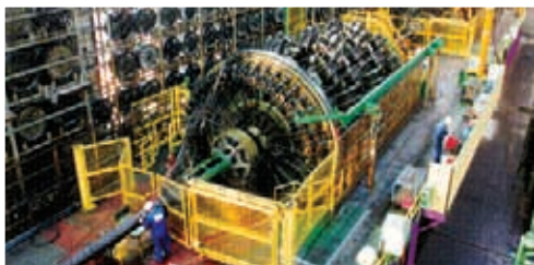
1. Flexible flowlines France Fabricated by Technip. Flexible riser flow lines will be used to connect the FPSO to the subsea equipment.
