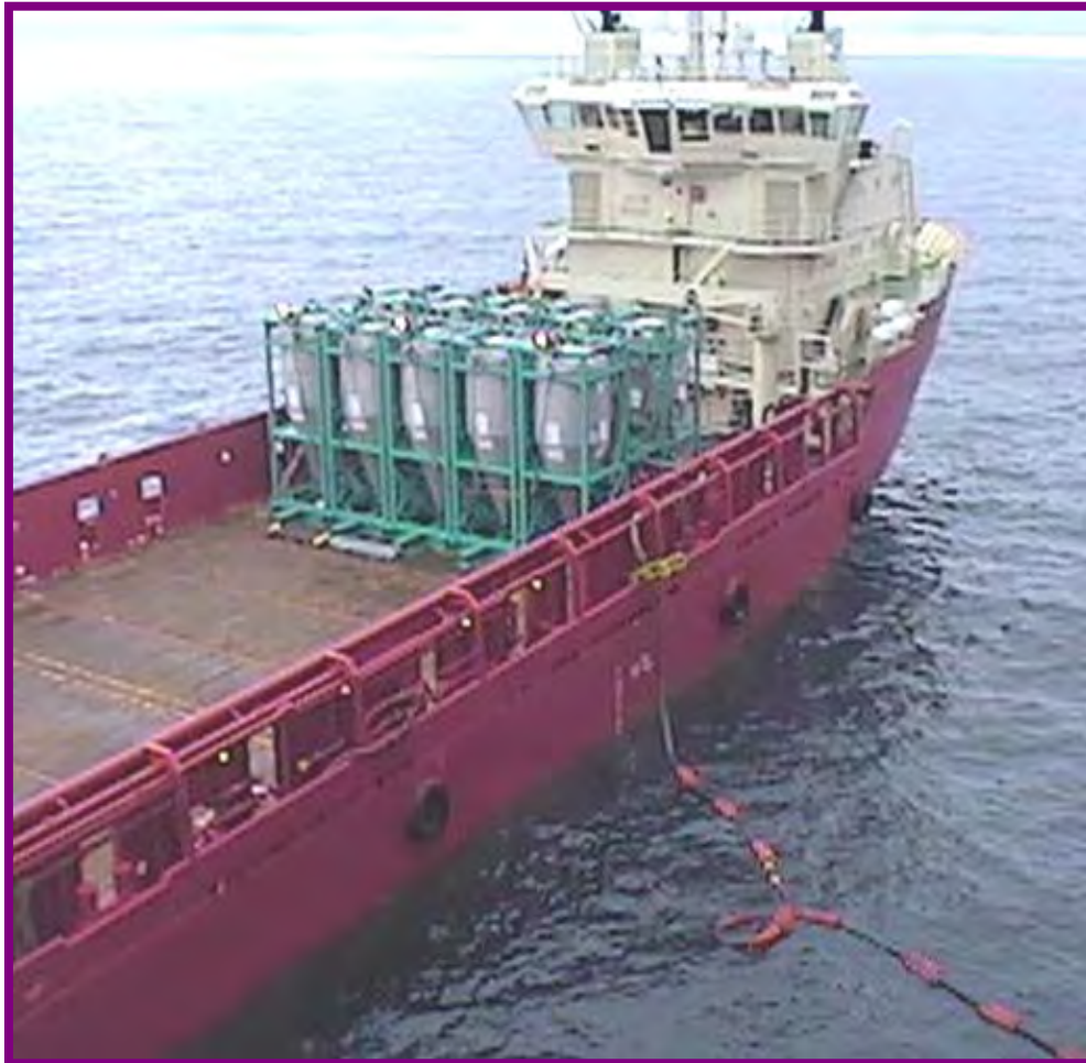
Figure A-3 Hose transfer of cuttings to bulk tanks on supply vessel
