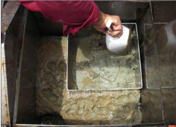
Image 1. Collection of deep water development area macrofaunal samples from an insert within the box core sample.
