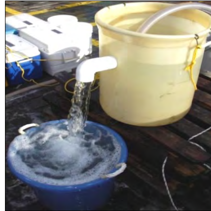
Image 2. Macroinfaunal sample sieving apparatus consisting of an upper holding barrel and lower spillover barrel.
