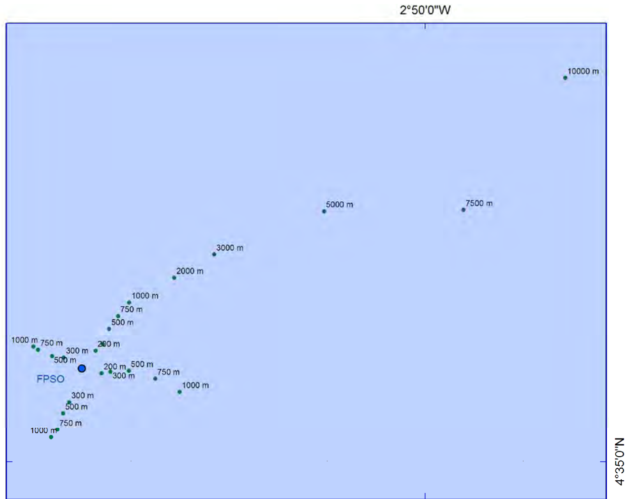
Figure 4.1a – Map indicating measurement sampling stations (●) during a normal FPSO operation. Guesstimated ranges are provided for each measurement point.
