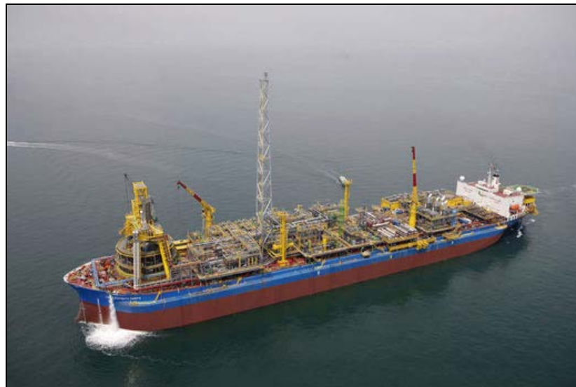
Figure 47. Example of operational overboard discharges from an FPSO (source: internet).
